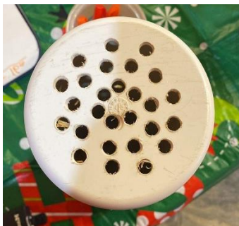
25 to 28 half inch holes drilled into a solid cap as the base
